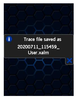
**FlashScan/AutoCal V3** maintain an internal buffer of the most recent messages sent to and received from the vehicle. That buffer is stored in RAM memory and is wiped clean each time the device is powered off or rebooted (and each time a trace file is saved). Therefore trace files can only be saved **before** powering off or rebooting the device which usually means before disconnecting from the vehicle.
